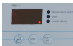
Display showing alarms turned on
